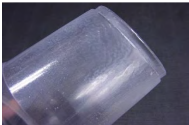
Pockmarked surface. Possible causes: rough plug surface, material sticking (XTL)
