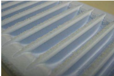
Pockmarked surface. Possible causes: rough plug surface, material sticking (XTL)
